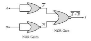
$\overline{A}$  and  $\overline{B}$  are the inputs for the last NOR gate. Hence, the output for the circuit can be written as:
