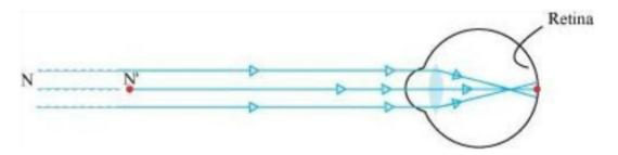
To correct this defect of vision, he must use a concave lens. The concave lens will bring the image back to the retina as shown in the given figure.
