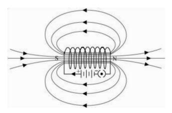
In the above figure, when the north pole of a bar magnet is brought near the end connected to the negative terminal of the battery, the solenoid repels the bar magnet. Since like poles repel each other, the end connected to the negative terminal of the battery behaves as the north pole of the
