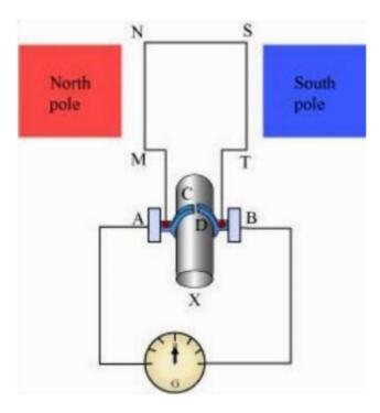
In this arrangement, brush A always remains in contact with the length of the coil that is moving up whereas brush B always remains in contact with the length that is moving down. The split rings C and D act as a commutator.
