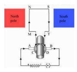
When a current is allowed to flow through the coil MNST by closing the switch, the coil starts rotating anti-clockwise. This happens because a downward force acts on length MN and at the same time, an upward force acts on length ST. As a result, the coil rotates anti-clockwise.
