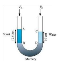
Height of the spirit column,  $h_1 = 12.5 \text{ cm} = 0.125 \text{ m}$
