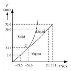
C is the triple point of the  $CO_2$  phase diagram. This means that at the temperature and pressure corresponding to this point (i.e., at  $-56.6^{\circ}$ C and 5.11 atm), the solid, liquid, and vaporous phases of  $CO_2$  co-exist in equilibrium.
