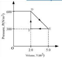
Its volume is then reduced to the original value from E to F by an isobaric process. Calculate the total work done by the gas from D to E to F
