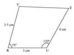
(2) Draw a line segment RU of 3 cm and an angle of 120° at point U. As vertex E is 4 cm away from vertex U, cut a line segment UE of 4 cm from this ray.
