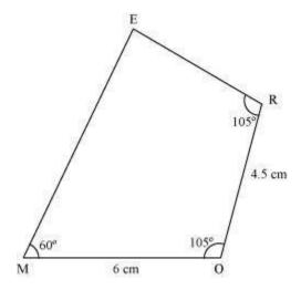
(2) Draw a line segment MO of 6 cm and an angle of 105° at point O. As vertex R is 4.5 cm away from the vertex O, cut a line segment OR of 4.5 cm from this ray.
