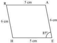
(2) Draw a line segment HE of 5 cm and an angle of 85° at point E. As vertex A is 6 cm away from vertex E, cut a line segment EA of 6 cm from this ray.
