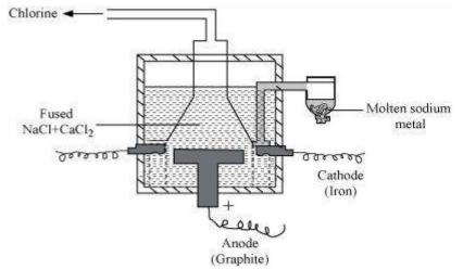
Steel is the cathode and a block of graphite acts as the anode. Metallic Na and Ca are formed at cathode. Molten sodium is taken out of the cell and collected over kerosene.
