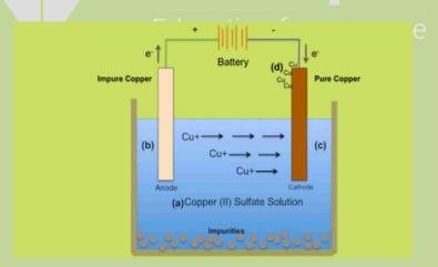
Cu<sup>++</sup>and SO<sub>4</sub> are present in the solution. When current passes through the solution, Cu++ ions move towards the cathode and the following reaction takes place at the cathode
