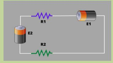
Let  $E_1 > E_2$  then the current flows in the anti-clockwise direction. Since the potential difference is equal to the work done on a unit positive charge or it is the gain or loss of energy when the charge is moving from one point to another point.
