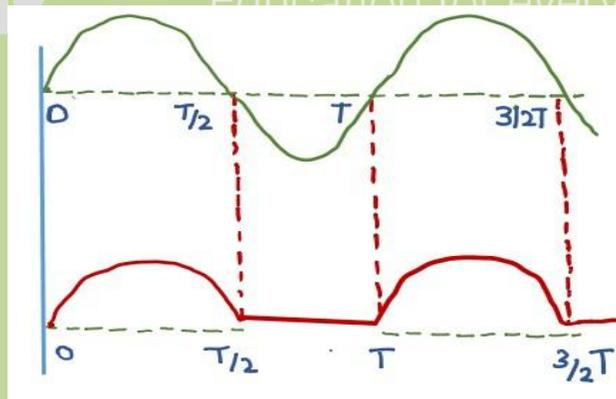
During the negative half cycle  $T/2$  to  $T$  the diode is reverse biased and it offers a very high resistance and no current flows through  $R$  and the potential difference across it almost zero.
