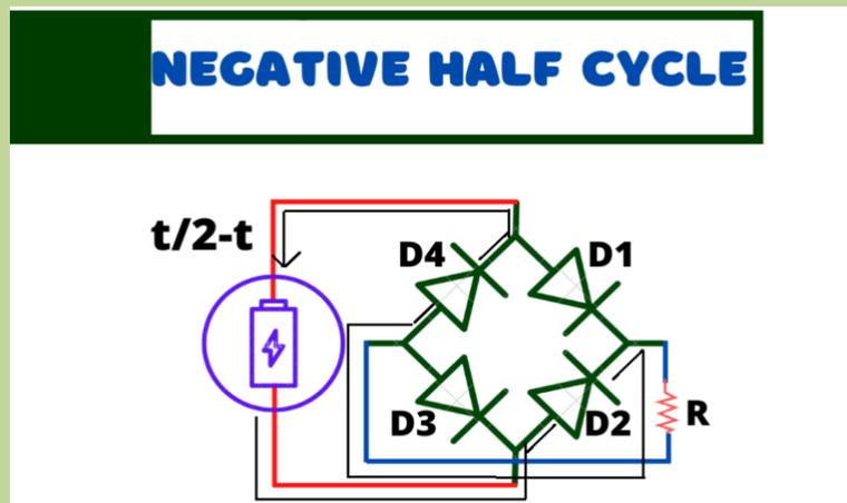
Therefore only  $D_2$  and  $D_4$  conducts. Now again the current flows from A to B through the load resistor in the same direction.
