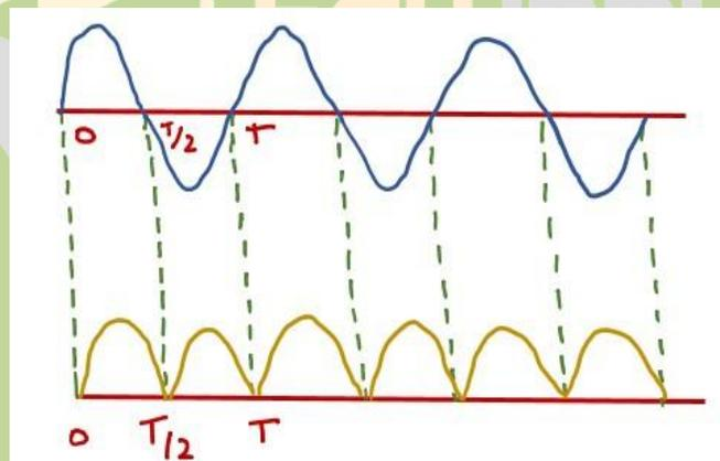
Therefore D.C output is obtained across the load. The output Voltage is not smooth but pulsating. It becomes smooth by using a circuit called (Combination of capacitors and inductors in the circuit as a filter).
