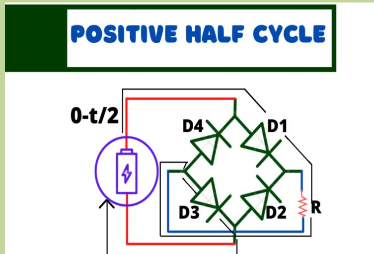
Therefore only diodes D<sub>1</sub> and D<sub>3</sub> conduct.
