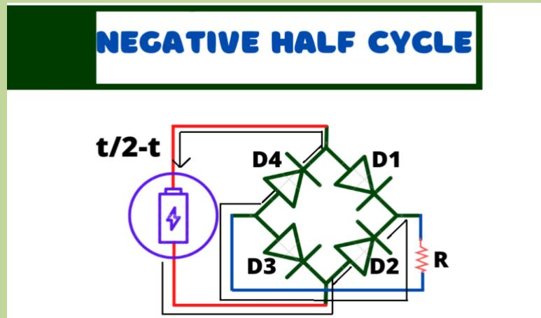
Therefore only D<sub>2</sub> and D<sub>4</sub> conducts. Now again the current flows from A to B through the load resistor in the same direction.
