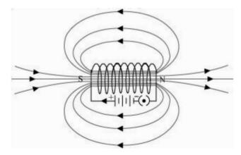
In the above figure, when the north pole of a bar magnet is brought near the end connected to the negative terminal of the battery, the solenoid repels the bar magnet. Since like poles repel each other, the end connected to the negative terminal of the battery behaves as the north pole of the
