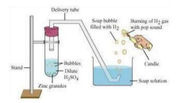
**Solution:-** Hydrogen gas is usually liberated when an acid reacts with a metal.
