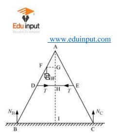
$N_{\rm B}$  = Force exerted on the ladder by the floor point B  $N_{\rm C}$  = Force exerted on the ladder by the floor point C
