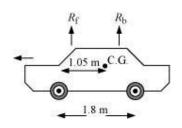
$R_{\rm f}$  and  $R_{\rm b}$  are the forces exerted by the level ground on the front and back wheels respectively.
