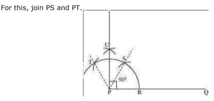
We have,  $\angle$  SPQ =  $\angle$  TPS = 60°. In (iii) and (iv) steps of this construction, PU was drawn as the bisector of  $\angle$  TPS.
