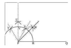
We have,  $\angle$  SPQ =  $\angle$  TPS = 60°. In (iii) and (iv) steps of this construction, PU was drawn as the bisector of  $\angle$  TPS.
