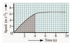
The shaded area which is equal to  $1/2 \times 4 \times 6 = 12$  m represents the distance travelled by the car in the first 4 s.
